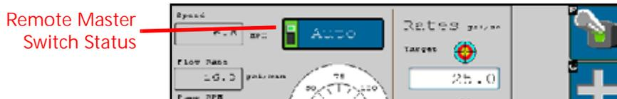
**NOTE:** Both the remote master (foot switch) and the master switch must be toggled on to apply product.
