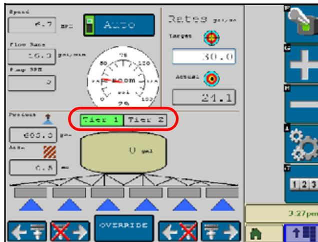
Above the tank volume display, a tiered boom status display will indicate tier 1 and tier 2 status. The tier stats will be displayed only if the tiered boom settings were entered. Refer to the *Tiered Boom Settings* section on page 24 for further information on setting up tiered booms.
