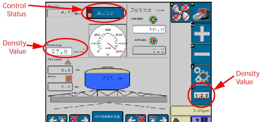
3. Select the control mode status area at the top of the main screen to toggle the control mode to manual.
